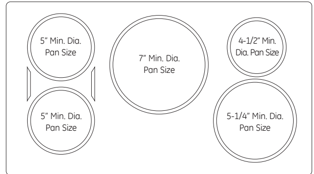
36" wide cooktop. Use the minimum recommended size pan shown for each cooking element.
